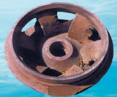
A METALLIC IMPELLER AFTER ONLY 3 MONTHS OF OPERATION IN FRESH WATER!
